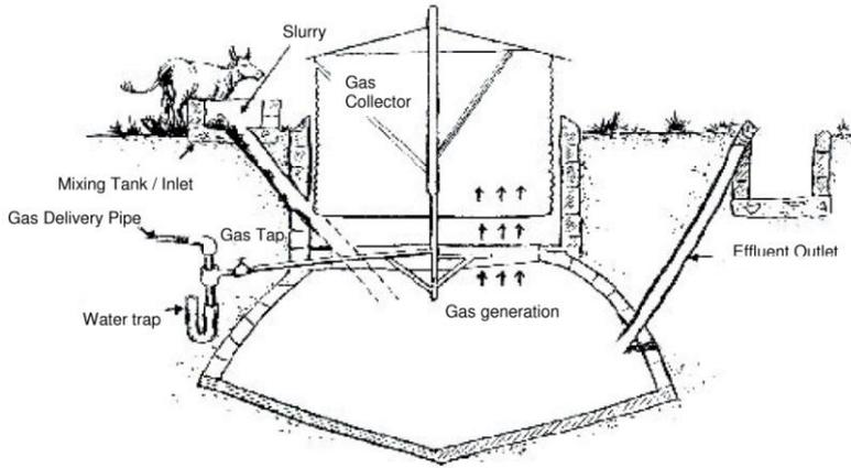
Figure 3: a typical floating cover biogas digester
