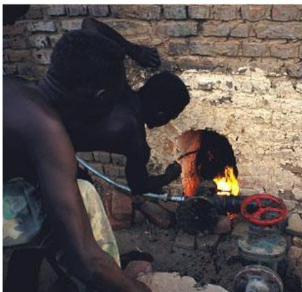
Figure 1: Brickmaker lighting a kiln with a liquid fuel burner. Photo:
