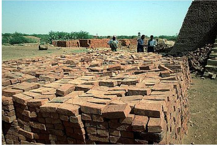
Figure 3: Pile of clay fired bricks with scotch kiln behind.
