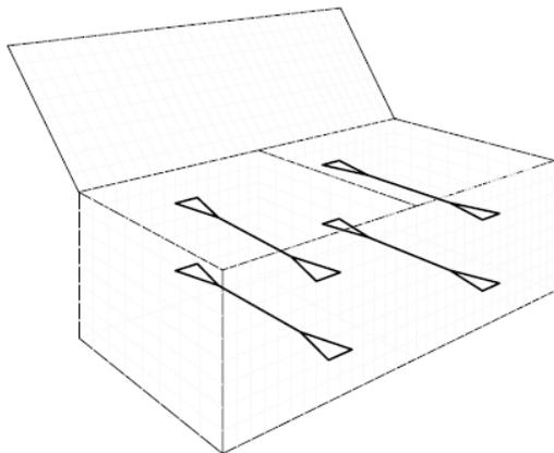
Figure 11: Cross links with wire
