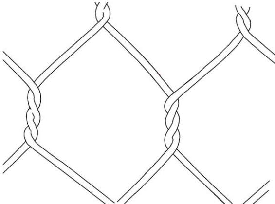
Figure 7: Hexagonal wire mesh with three twists.
