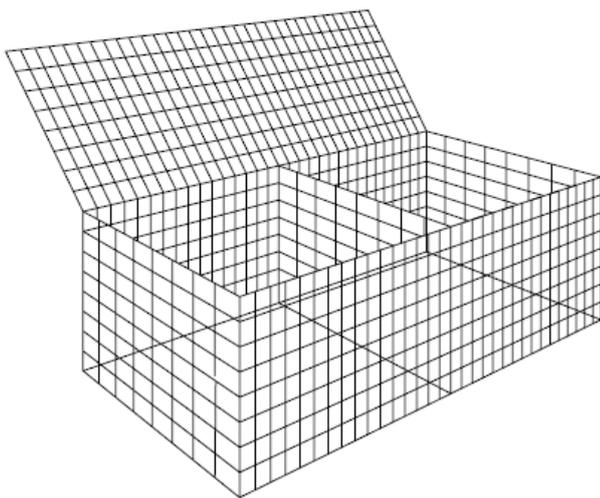
Figure 6: A basic gabion before loading with stones
