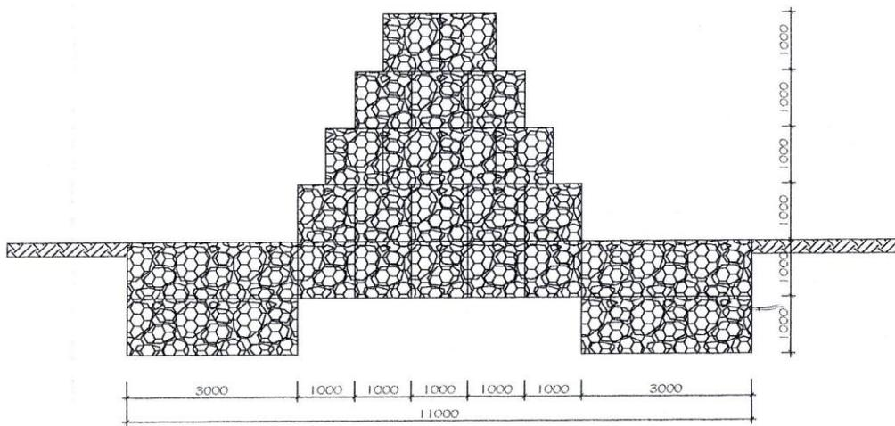
Figure 4: Cross section of a spur design in Chitwan showing substantial groundwork
