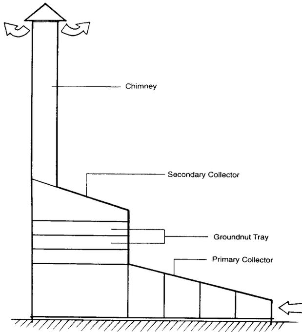
Figure 3: Indirect solar dryer
