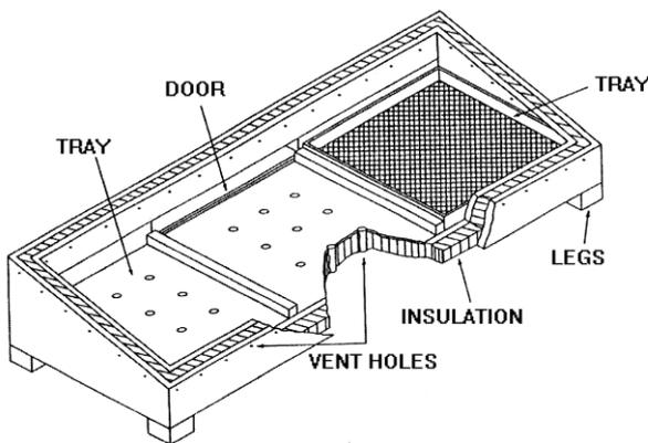
Figure 2: Typical brace type dryer
