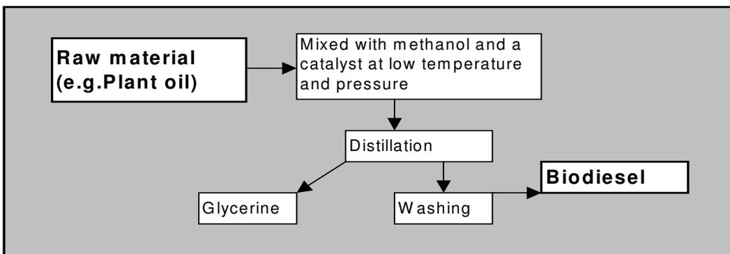
The raw oil is reacted with an excess of alcohol (often methanol or ethanol) in the presence of a catalyst (often potassium or sodium hydroxide). The products of this reaction are crude biodiesel and crude glycerine, with an excess alcohol, which is recovered and re-used.
