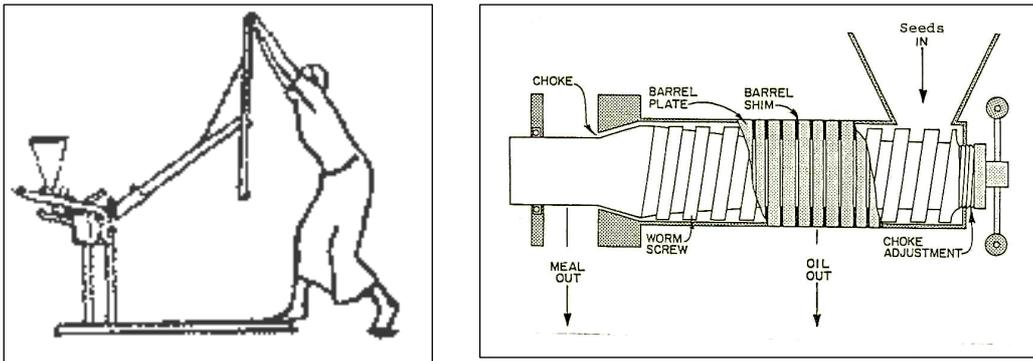
Plant oils can be extracted using hand tools, such as the Approtech oil expeller shown on the left (Approtech), or the motorised Sundhara-type oil presses, such as the one shown on the right (<http://www.jatropha.de/expellers/>).
