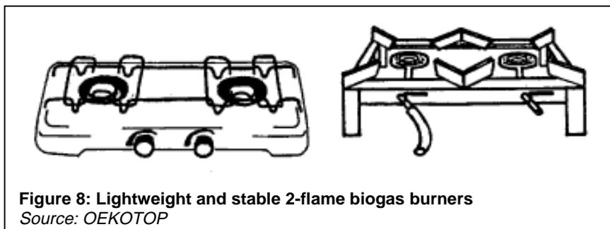
**Figure 8: Lightweight and stable 2-flame biogas burners**
