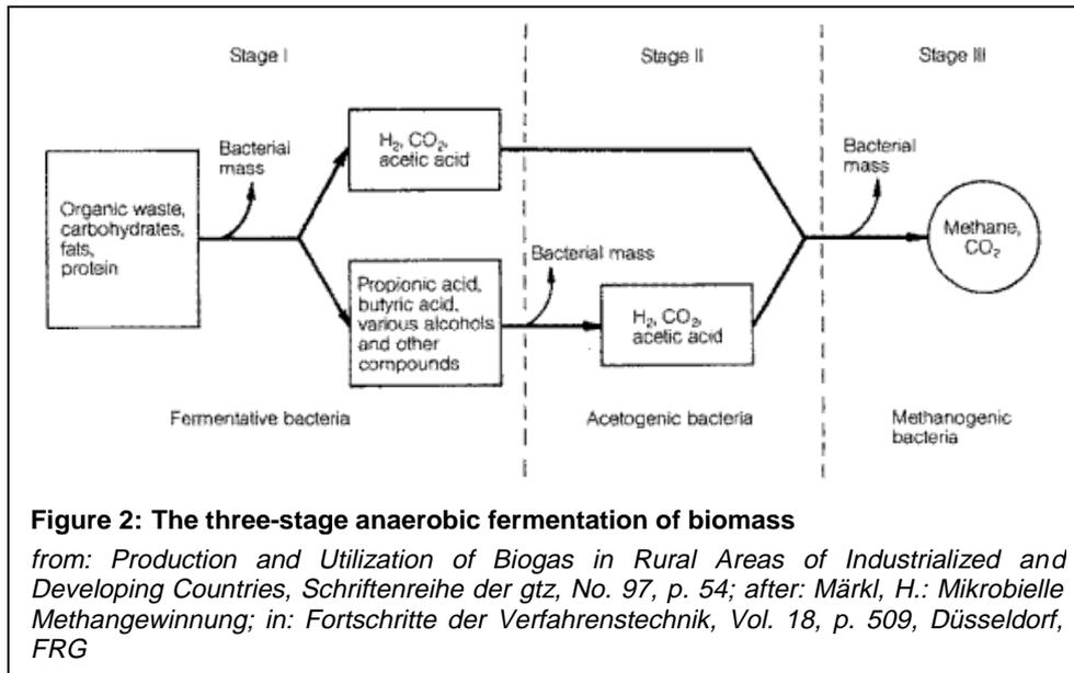
**Figure 2: The three-stage anaerobic fermentation of biomass**
