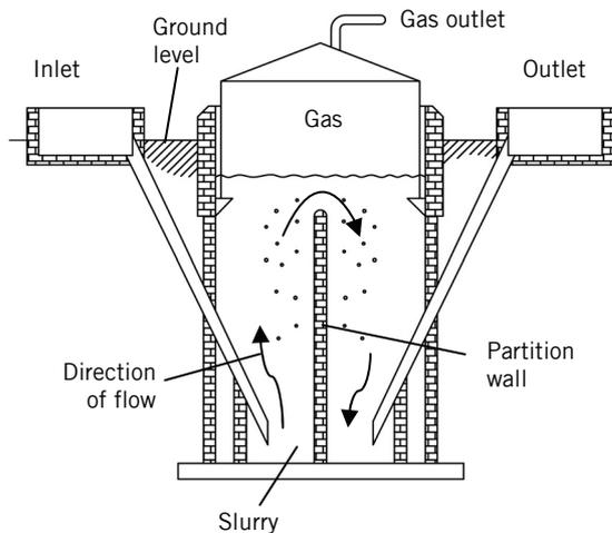
Figure 2: Floating cover digester
