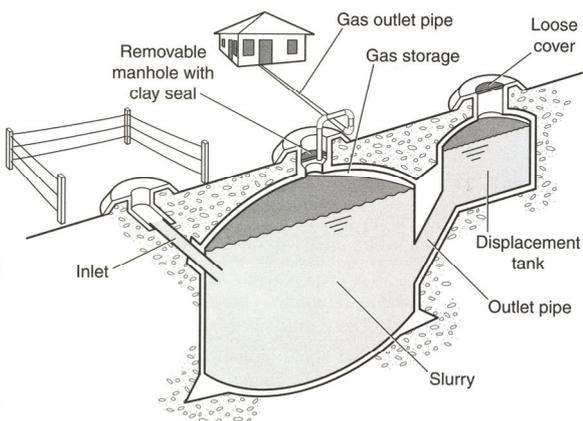
Figure 1: Fixed dome digester
