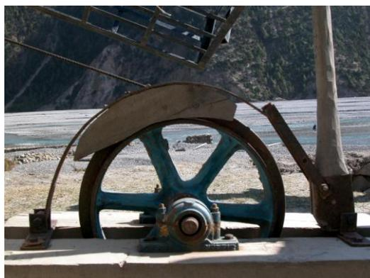
A typical braking system
