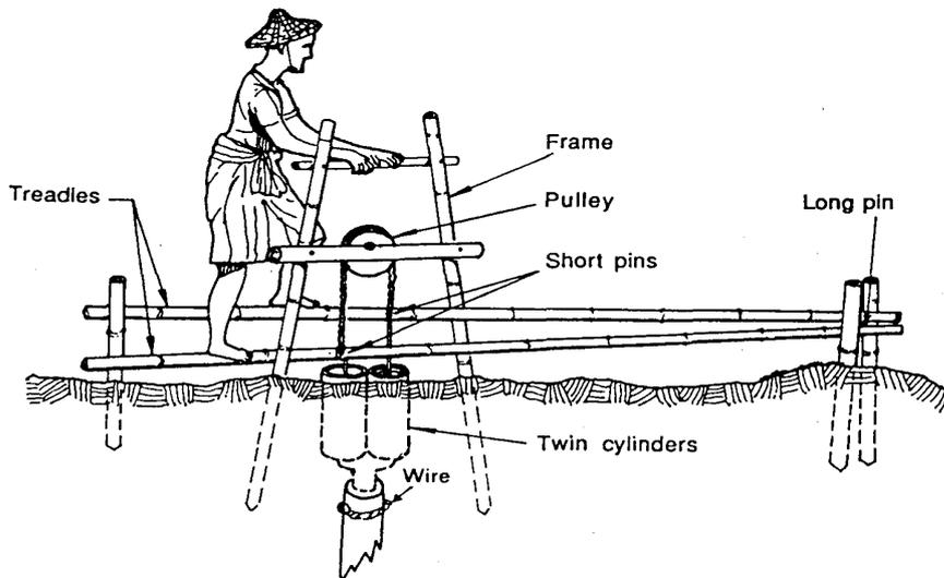
Figure 7: Treadle pump
