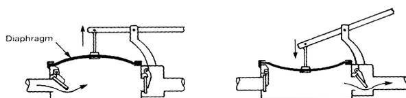
Figure 10: Diaphragm pump
