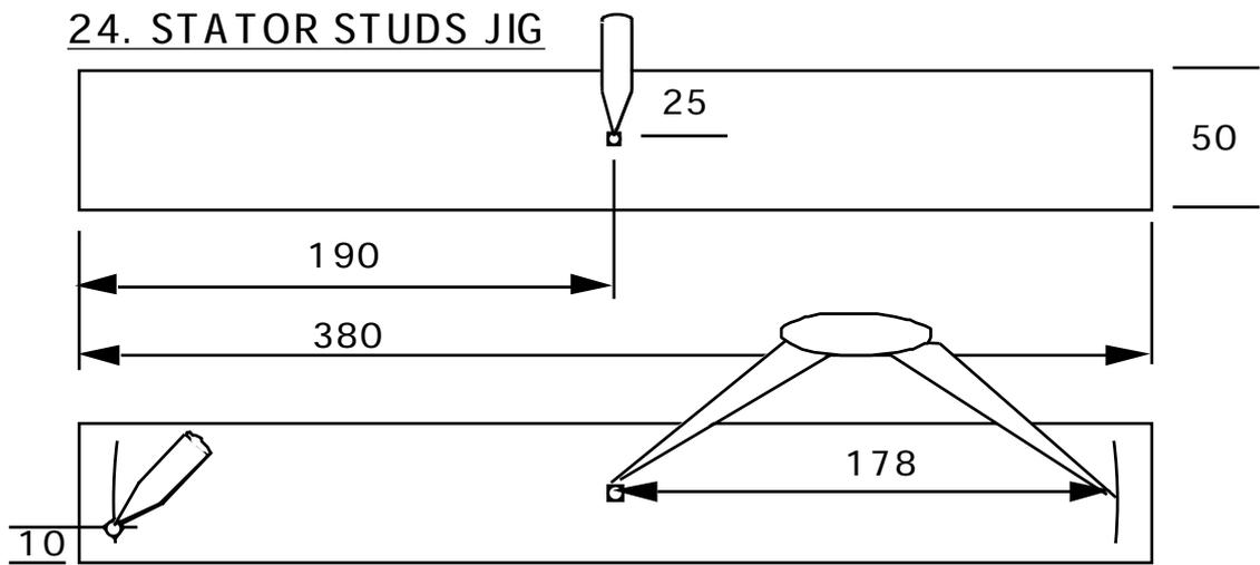
DRILL HOLES WITH A PILLAR DRILL FOR ACCURATE ALIGNMENT
