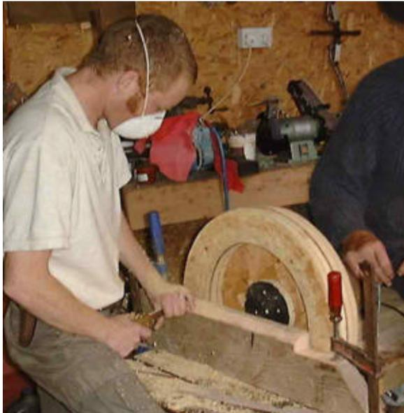
Turning a stator mould on an electric motor
