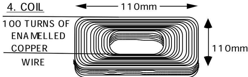
The coils will be wound on a plywood coil-former.
