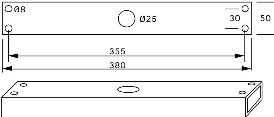
Weld the shaft in the 25mm hole. Take care to hold the shaft as square as possible (90 degrees) to the spine, when welding it.
