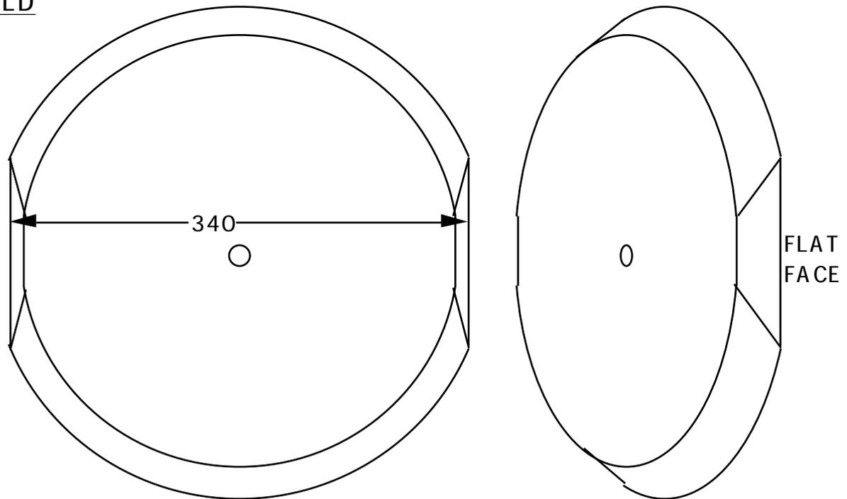
These two faces will create a thicker casting around the mounting studs.
