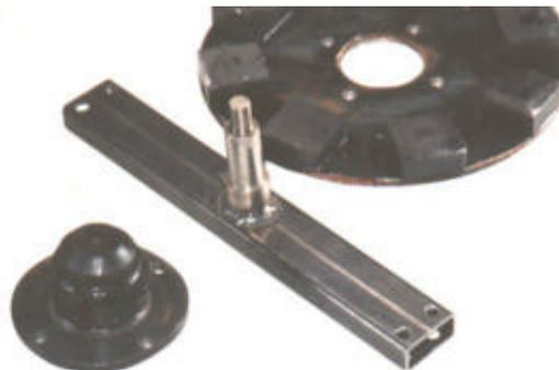
Spine, shaft, hub and magnet rotor
