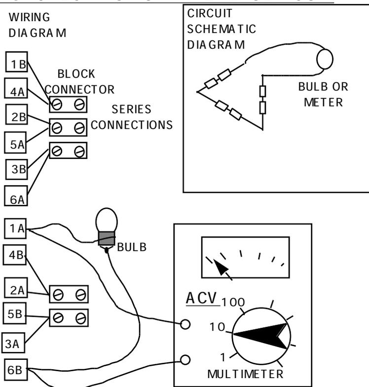
There will always be a small voltage in this test, because the coils are not perfectly positioned in the mould. If the test gives more than one volt, then it should be possible in future to make a better stator by placing the coils at exactly equal distances apart in the mould.
