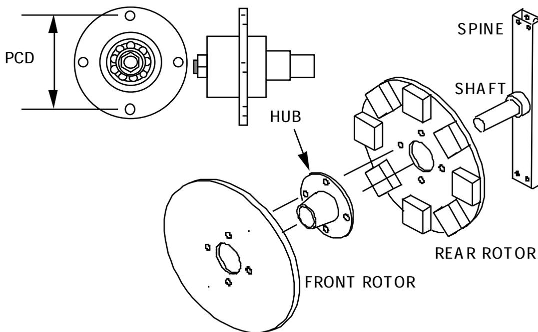
The PCD jig will be used to drill holes in the rotors etc.
