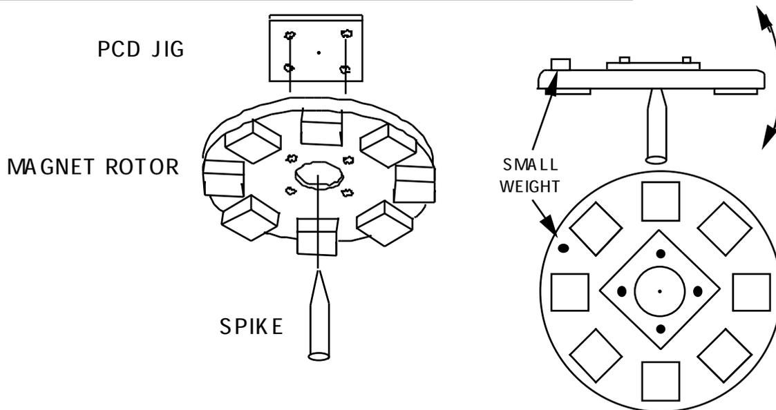
If the rotor will sit level, then it is balanced. If it will not sit level, then add small weights to it, or drill out some of the resin between magnets, until it will sit level. Turn the PCD jig around on the rotor, and check it again. Replace any weights with pieces of M10 threaded rod, screwed into holes in the resin between the magnets.
