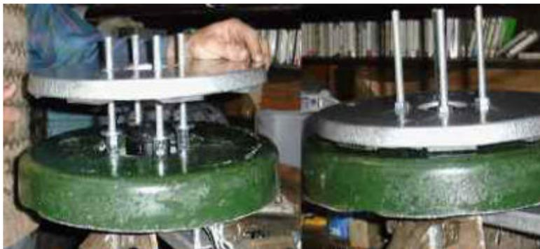
Fitting the front magnet rotor
