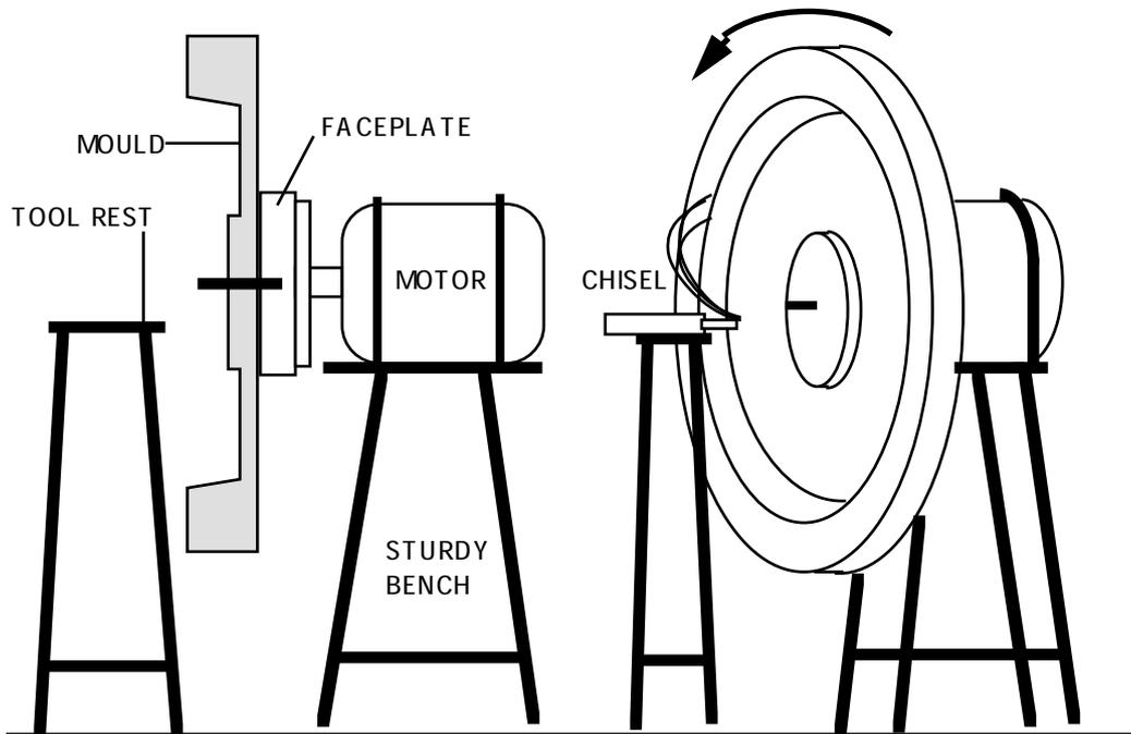
Now it is possible to shape the mould with a chisel. Wear a mask over your mouth to avoid inhaling the dust. Beware of loose clothing, which may become caught in the rotating mould.
