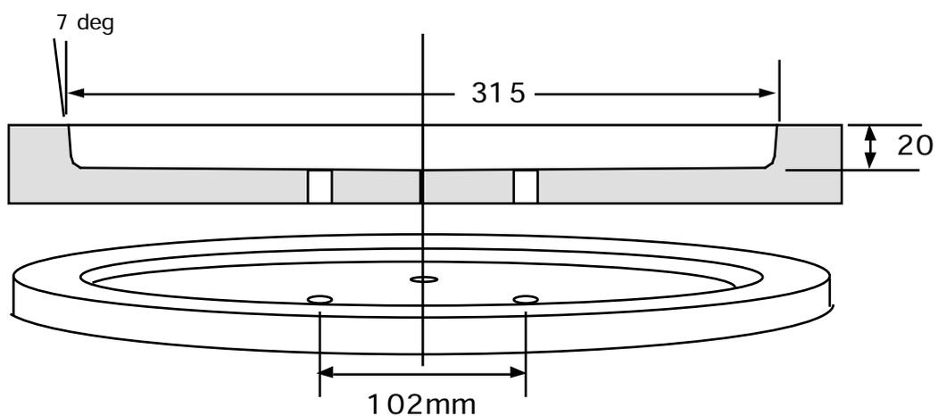
Use the PCD jig to drill four holes to match the holes in the magnet disks.
