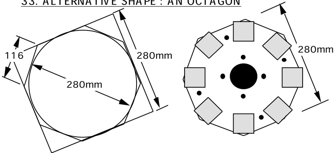
The central hole is made with a hole-saw or it can be cut out on a lathe.
