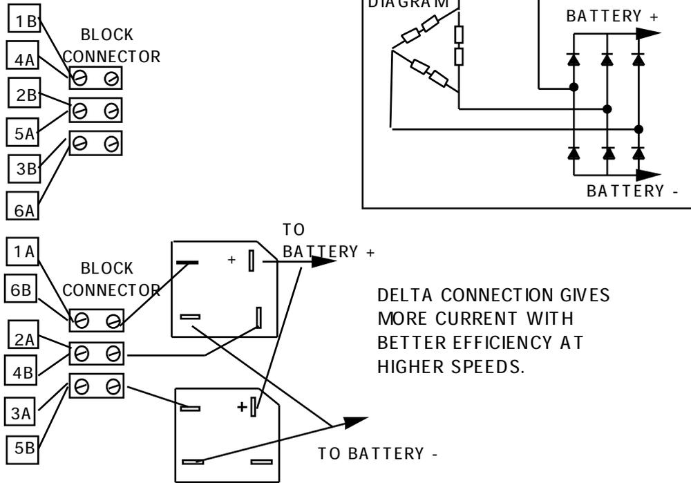
It is also possible to wire a relay (see diagram 48) which will switch the connections from star to delta and back as desired.
