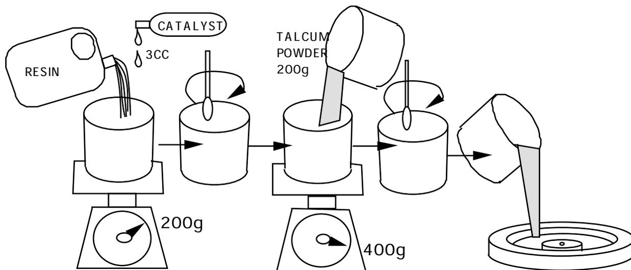
Mix resin with catalyst thoroughly but slowly to avoid churning in air bubbles. Add any talcum powder only after the catalyst is mixed. When the resin is mixed, use it at once. After a few minutes in the mixing bucket, it will heat up, and begin to set.
