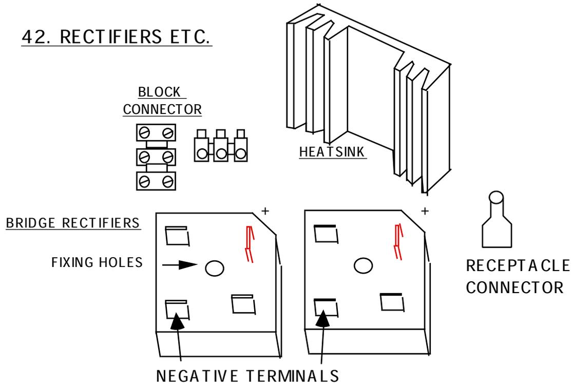
'Block connectors' are useful for connecting the wires from the stator. Alternatively soldering or crimping would be fine.
