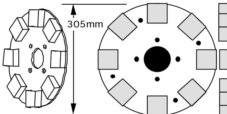
The magnet plates must be flat, not warped. It is not easy to cut the outer circle without warping the plate. A guillotine can cut steel plate into an octagon (see diagram 33), without warping the plate. This is an alternative way to make the rotor disk. First cut a square, draw a circle on it, and then cut off the corners at 45 degrees. The length of each edge is 116 mm.
