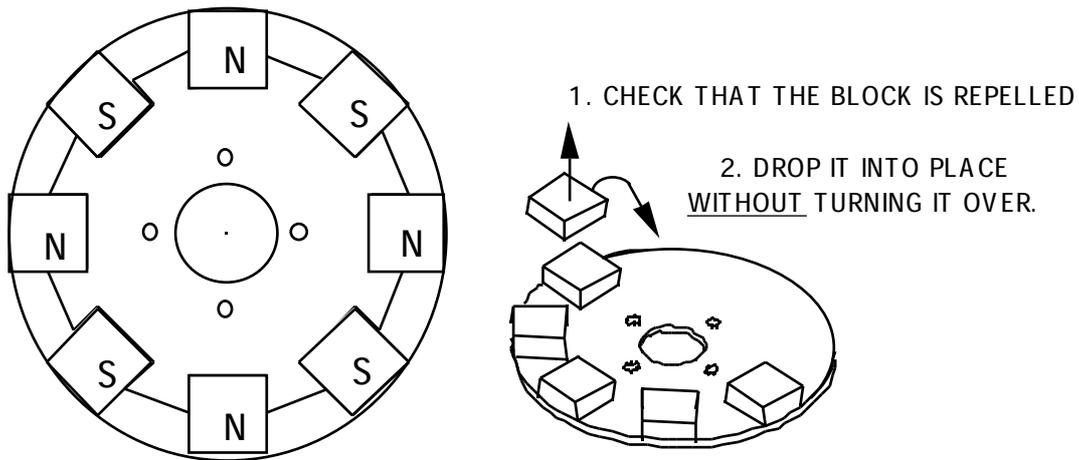
The two magnet rotors must attract each other when the mounting holes are aligned. Check that the magnets next to the holes on one rotor are different from the ones next to the holes on the other rotor (see diagram 36).
