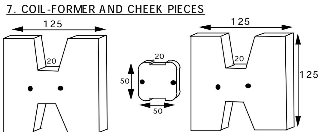
The coil former is 50mm by 50mm by 13 thick. It has rounded corners. The two 'cheek pieces' are 125mm by 125mm. There are 20mm wide notches top and bottom in each. The notches are for putting masking tape under the coil, so that it can be taped up before removing it from the former.
