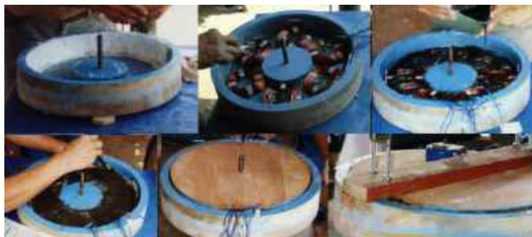
Six stages of the rotor casting procedure
