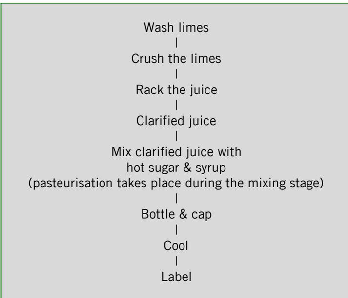
Lime juice is very acidic and it is important that workers are provided with protective gloves to avoid damage to the hands. Only inert materials can be used to process lime juice as it will rapidly corrode steel. Stainless steel, plastic, glass and wood are recommended.
