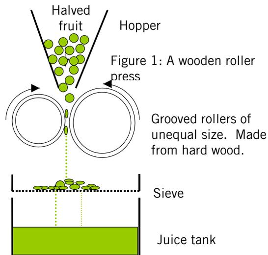
length and rotate inwards powered either by hand or electric motor. One roller is of a slightly larger diameter than the other which provides a shearing action as the fruit passes through. The gap between the rollers can be adjusted and maintained by heavy springs.
