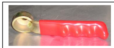
Fig. 5. Different types of Crown cappers Photo from Peter Fellows
