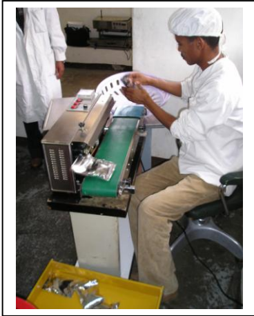
Fig. 11. Band sealer for plastic film Photo from Peter Fellows
