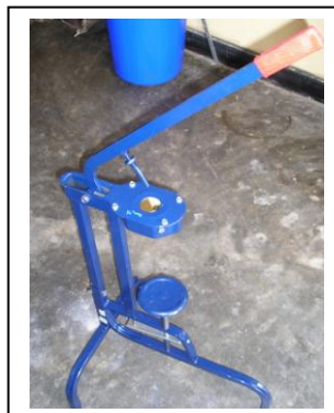
Fig.7. Manual 'Omnia' capper
