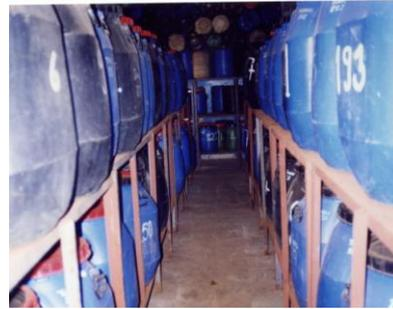
Fig 1: Polypropylene drums used as shipping containers for fruit pulp (Photo: Peter Fellows)
