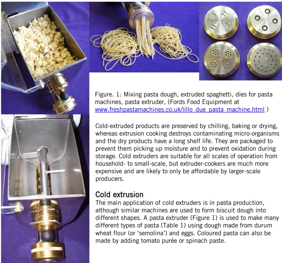
Figure. 1: Mixing pasta dough, extruded spaghetti, dies for pasta machines, pasta extruder, (Fords Food Equipment at [www.freshpastamachines.co.uk/lillo\\_due\\_pasta\\_machine.html](http://www.freshpastamachines.co.uk/lillo_due_pasta_machine.html) )
