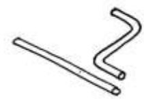
**Bottom Fuller** – Normally used with a top filler, to create rounds or indents in material.
