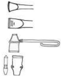
**Hot Chisel** – Used for cutting hot metal, by striking with a hammer. This tool is not hardened and should not be used to cut cold material, only heated.
