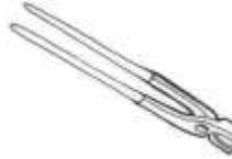
**Tongs** – Used to hold material when it has been heated and is ready for work. These can be made in the forge, for different pieces of work. The heads can be shaped to grip different sizes and shapes of material.
