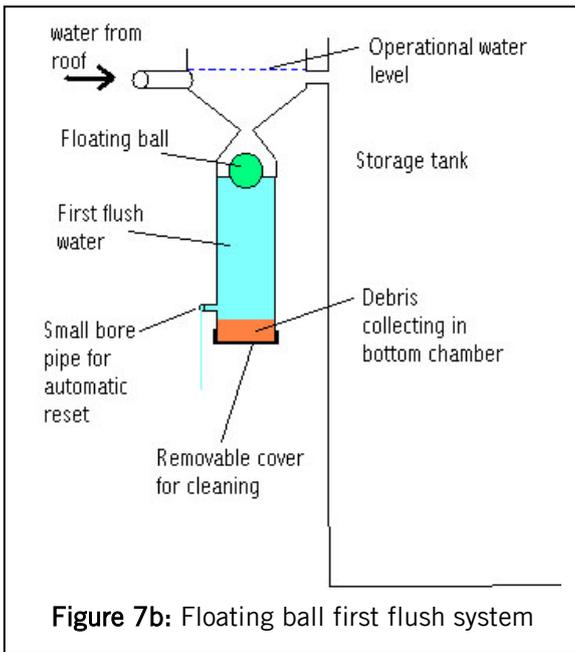
**Figure 7b:** Floating ball first flush system
