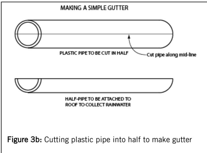
Figure 3b: Cutting plastic pipe into half to make gutter
