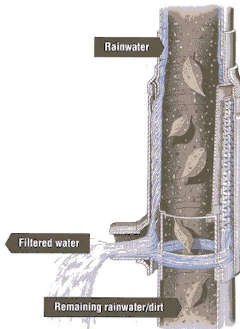
**Figure 8 :** the WISY filter (downpipe and high-capacity below ground versions)
