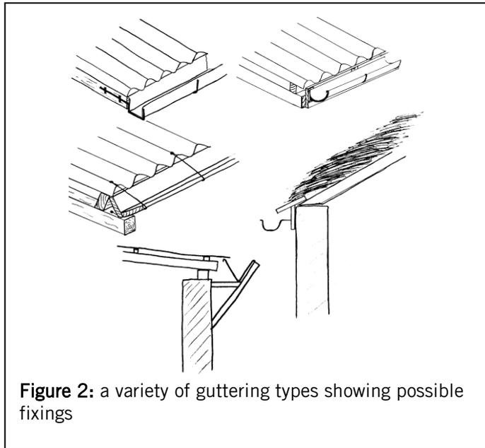
Figure 2: a variety of guttering types showing possible fixings
