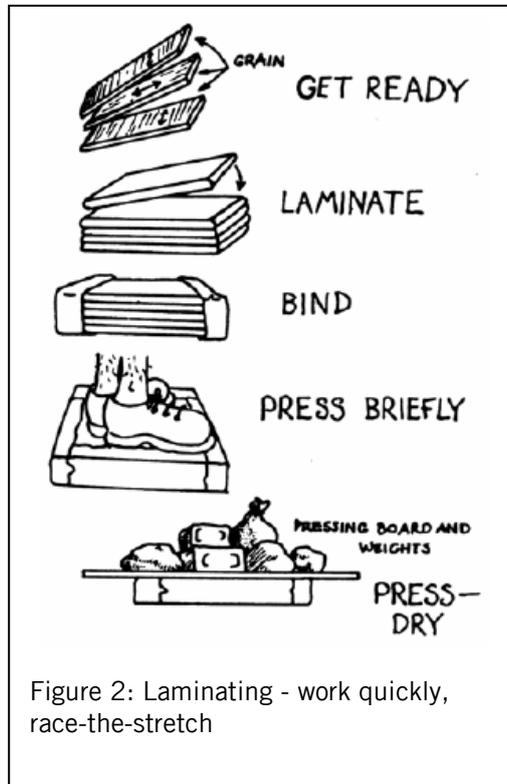
Figure 2: Laminating - work quickly, race-the-stretch
